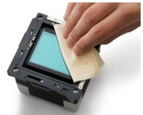
The special Green Clean cleaning liquid does not contain alcohol or aggressive cleaning substances, but is able to dissolve fatty/oily substances and other residual dirt. It is important that the cleaning liquid does not dissolve instantly, as do alcohol based products, but that they evaporate slowly do give enough time for the „Silky Wipe“ to spread the liquid and dissolve all dirt before evaporation and absorption into the cloth.
